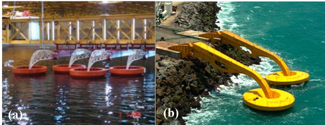
Figure 19. COPPE hyperbaric wave converter: (a) medium-scale model with a ratio of 1:10 at LabOceano [187]; (b) installed full-scale prototype.
