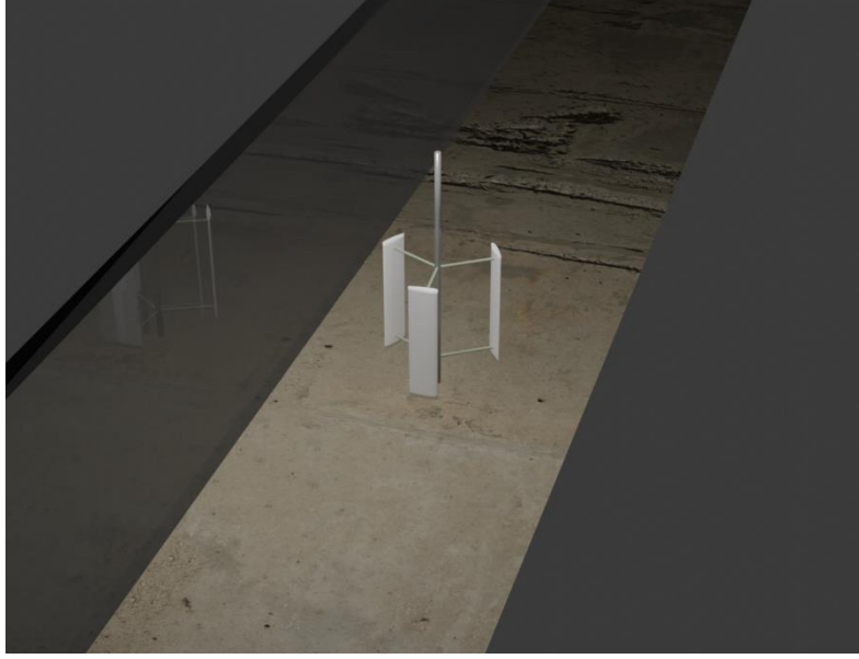
Fig. 1. Illustration showing the flume and the designed VAT based on the experiments.
