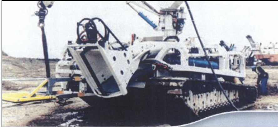
Plate 2.11 Typical specialist cable burial ROV
