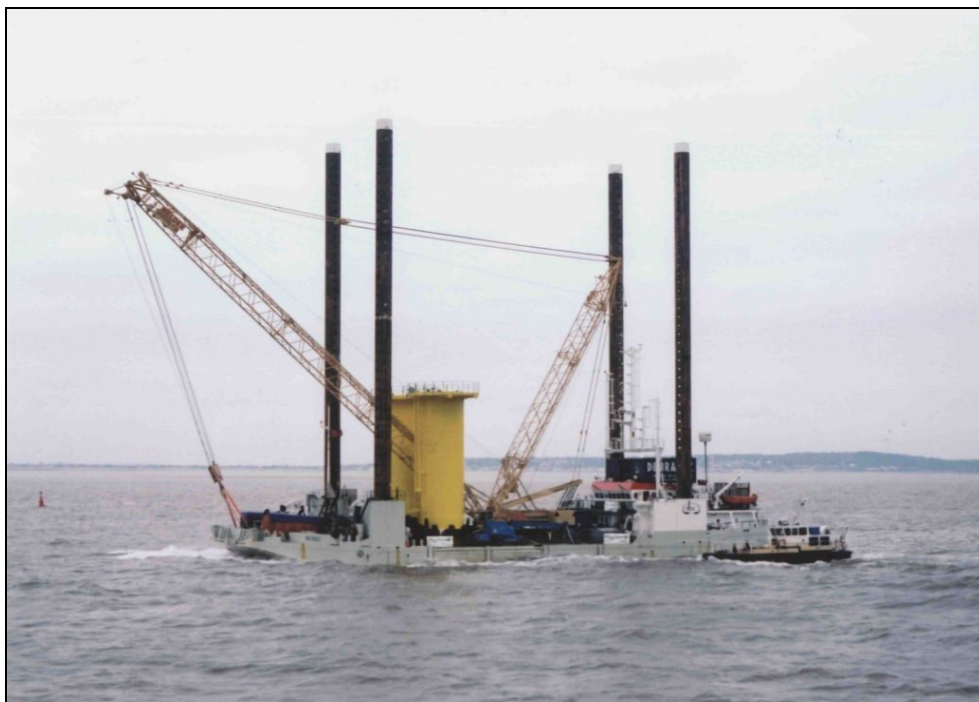
Plate 2.6 Transition pieces in transit to the offshore work site
