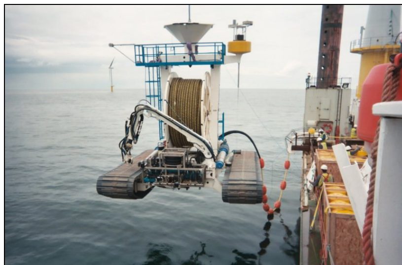
Plate 2.12 Example of a tracked ROV with dedicated cable reel for simultaneous cable lay and burial operations
