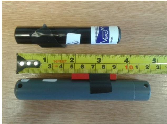
**Figure 7:** VEMCO V16P-6H continuous transmitter tag.
