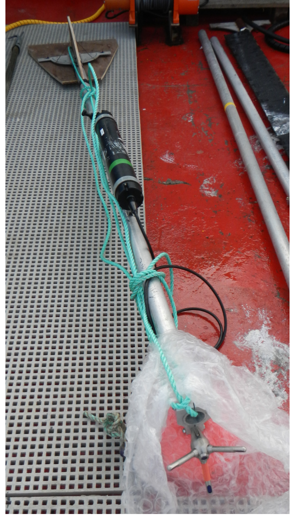
Fig. 7. Photo of the ADV fixed to the glider on the deck of the barge. The probe head is still wrapped in bubble wrap for protection.
