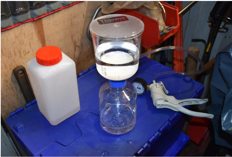
Figure 5. eDNA filtration set-up on the research vessel during the T-1.
