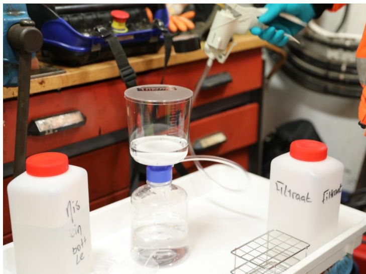
Figure 2-10: eDNA filtration set-up on the research vessel.
