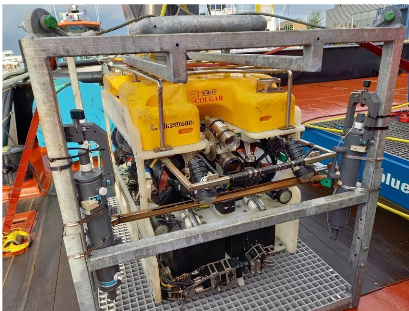
Figure 2-9: ROV in cage, with 2 Niskin bottles attached vertically.
