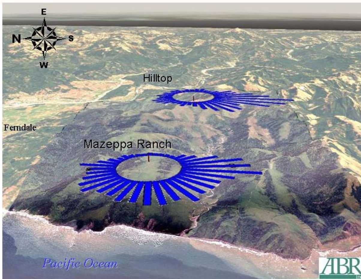
Figure 7. Map of the study site with flight directions of radar targets during the primary sampling period (16 April–30 May) at the Hilltop and Mazeppa Ranch stations at the proposed Bear River Windpark, California, spring 2007. Elevation of topographical features were doubled to enhance the three-dimensional perspective.
