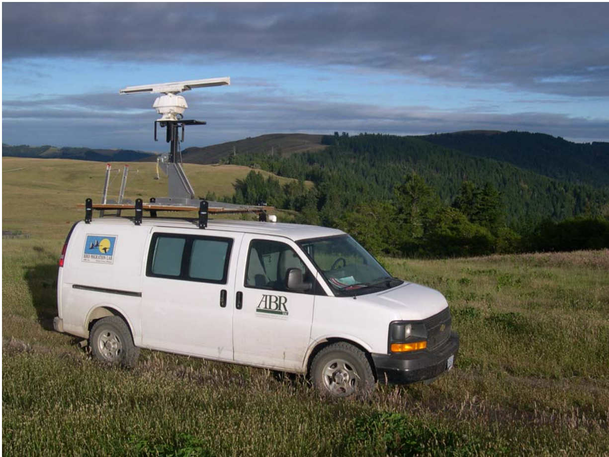
Figure 2. Mobile radar lab at Bear River Ridge with radar in surveillance position.
