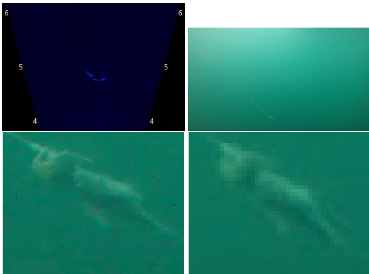
Figure 20: TOP-LEFT: Aris image of the target (shackle with line to a 20 cm herring) at 4.5 m range. TOP-RIGHT: GOPRO image ( 3840 \times 2160 pixels) showing the target at 3.3 m range. BOTTOM-LEFT: Zooming in on the 20 cm herring, full resolution of the GOPRO. BOTTOM-RIGHT: Same image as to the left, except that the pixel size is increased by a factor of 2. Measurements were made at 1912 UTC on 23 October 2018.
