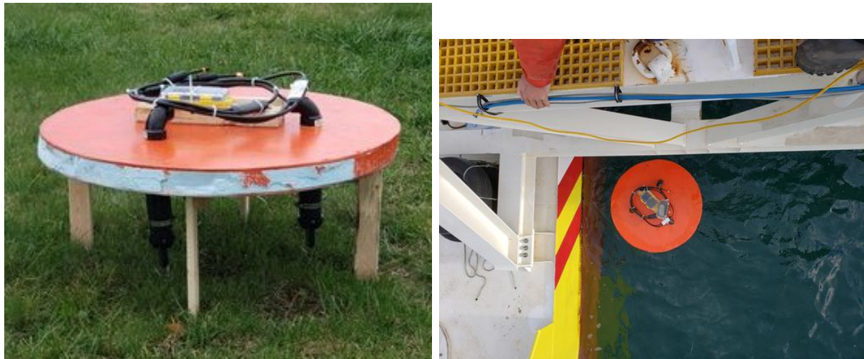
Figure 36: LEFT: Pad-float hydrophone-array on a wooden stand, showing Smart Cable and GPS/compass above and hydrophones below. RIGHT: Deployed and passing between the hulls of PLAT-I. Photo credit: Mike Adams.
