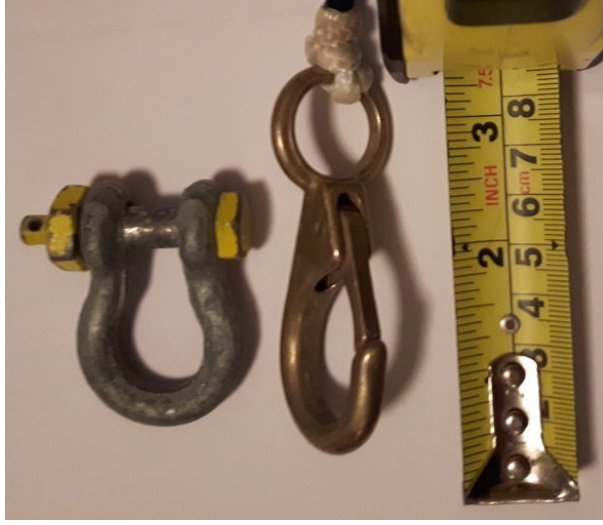
Figure 3: Shackle and brass clip: Brass clips were used on the cross-line for the target float on 13 October 2018. The shackle was used to weight targets that were cast from PLAT-I on 23 October 2018. Photo credit: Connor Sanderson.
