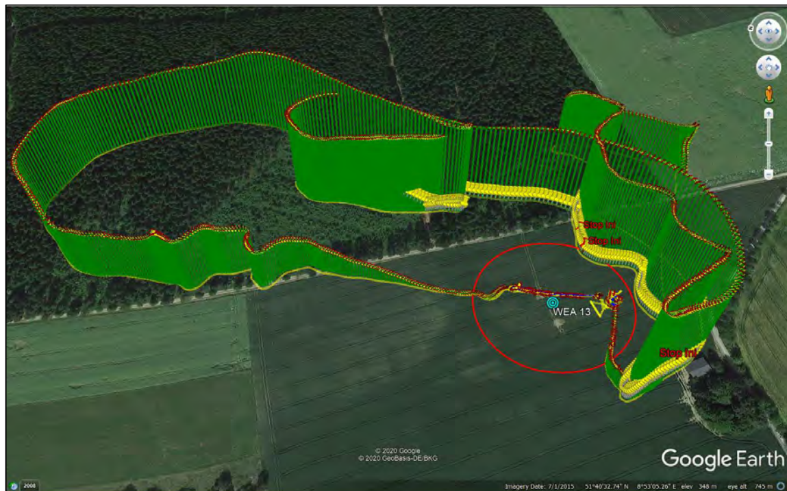
Figure 7 Robird drone and SafeWind comparison (green – flight track of Robird drone; yellow pin – matching SafeWind videos; red pin – shutdown initiation; red circle – wind turbine rotor area; light blue circle – position of WEA 13)
