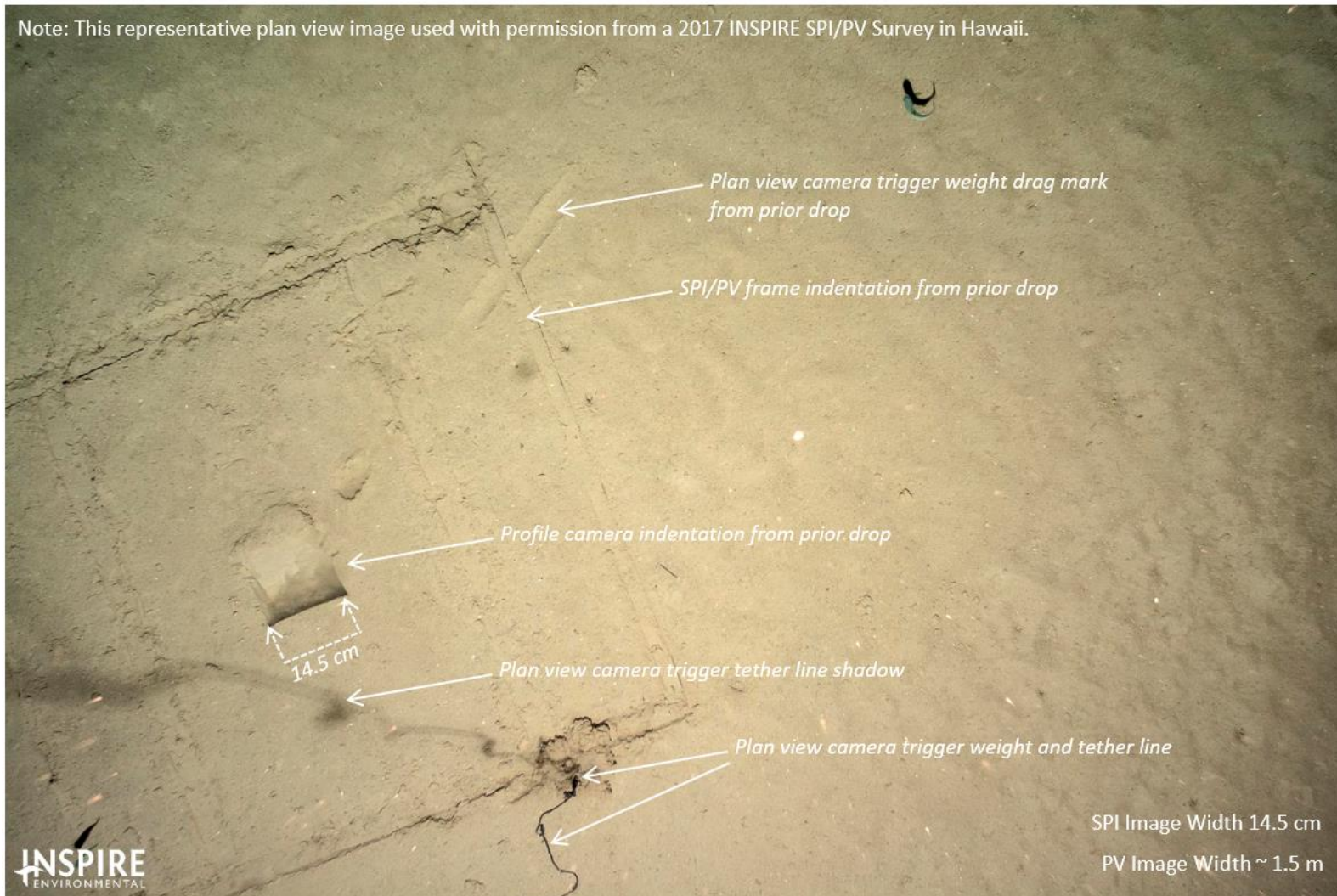
Figure 2.4-2 This representative plan view image shows the sampling relationship between plan view and sediment profile images. Note: plan view images differ between surveys and stations and the area covered by each plan view image may vary slightly between images and stations.
