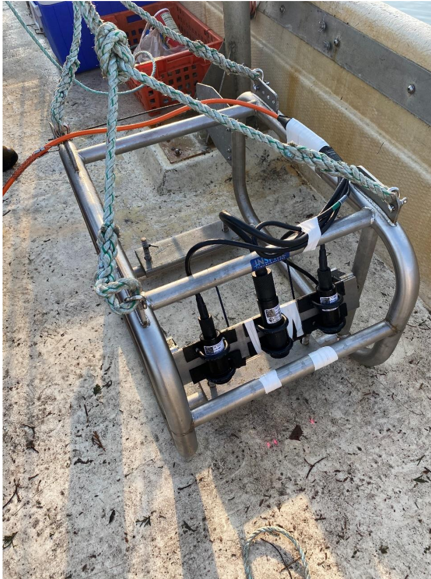
Figure 2.3-1 Photographs of the video sled used during the ICW survey to collect video footage in order to detect the presence and extent of submerged aquatic vegetation (SAV) within 100 m of the planned HDD route
