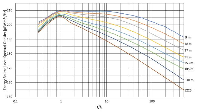
Figure 7. Energy source level spectral density curves for underwater explosion events at various depths expressed in normalized frequency, relative to the frequency  $f_{b1}$  of the first bubble pulse (after Urick 1983).
