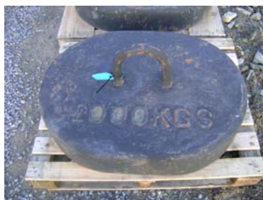
1 tonne steel clump weight 1.08m W x 0.84m D x 0.20m H
