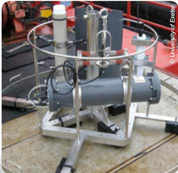
Static hydrophone which can be deployed underwater to measure ambient noise
