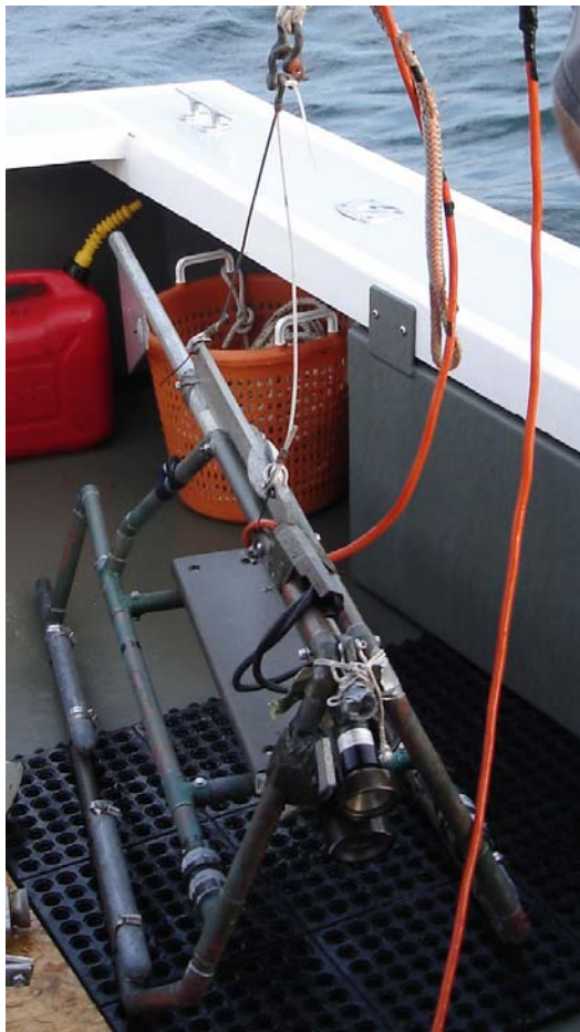
Figure 2. Simrad OE9030/9031 Diver Television System
