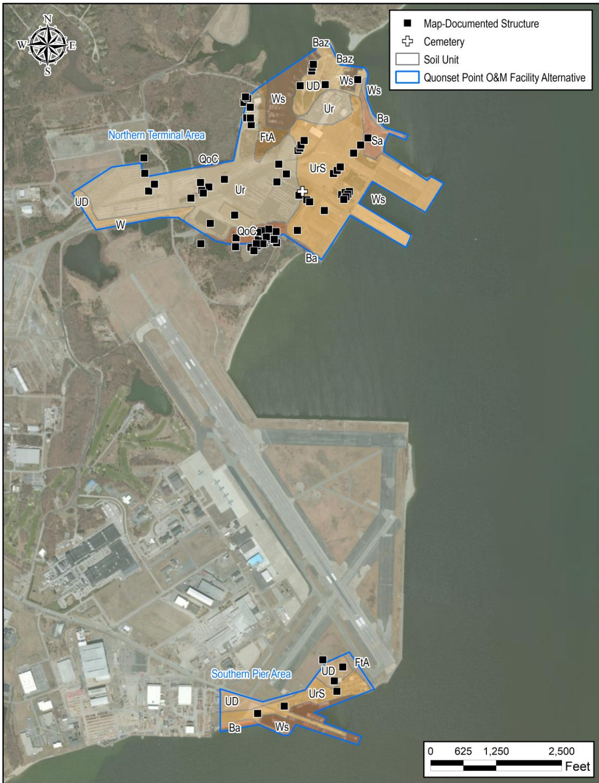
Inset 2.1-2. Map-Documented Structures and Soil Units within the Quonset Point O&M Facility Site.
