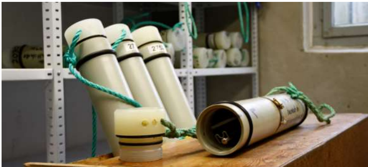
Figure 4.2 C-PODs: left: ready for deployment; right: opened C-POD.
