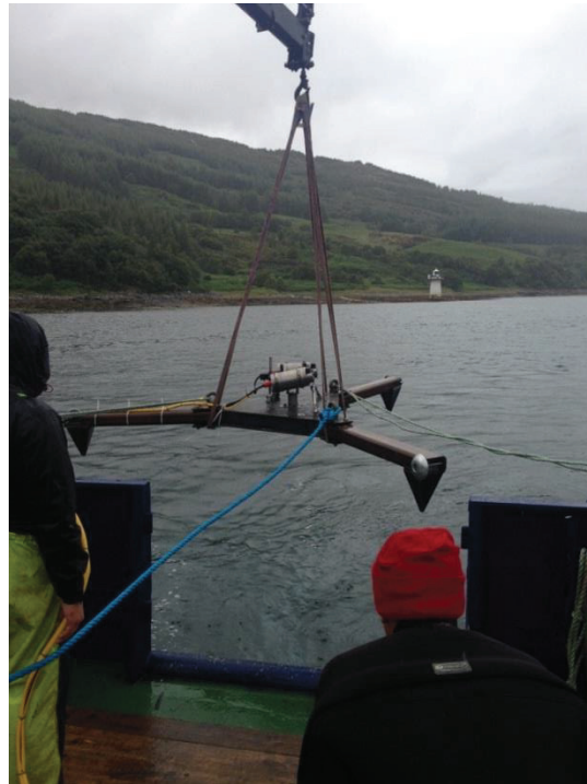
Figure 38: Hi Current Underwater Platform (HiCUP) with dual sonar configuration in Kyle Rhea. The left panel shows the location of the HiCUP in the channel and the right panel shows it being deployed from the survey vessel.
