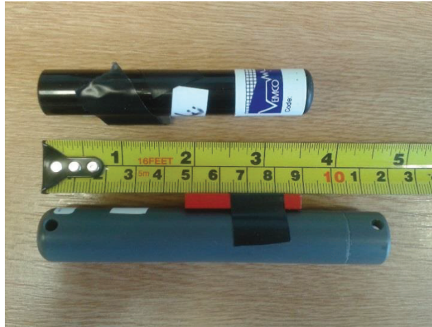
Figure 7: VEMCO V16P-6H continuous transmitter tag.
