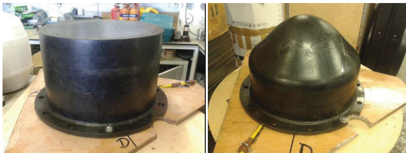
Figure 6: Polyethylene cowlings, on a plywood base, used to protect the two hydrophone clusters.
