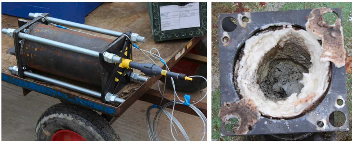
Fig. 3. Left: a photograph of a 10 kg shell showing the 25 g shaped charge used to initiate deflagration. Right: a photograph of the shell and contents after deflagration (white and grey matter around inner edge of shell).
