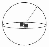
(ii) Signals from two satellites can be used to locate the receiver on a circle that is the intersection of two spheres.
