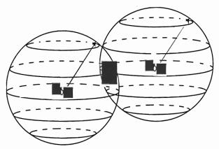
(iii) Data from three satellites can be used to locate the receiver at either of two points.
