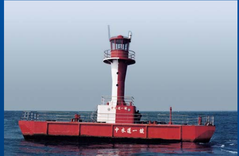
100 W wave power device used in navigation ship
