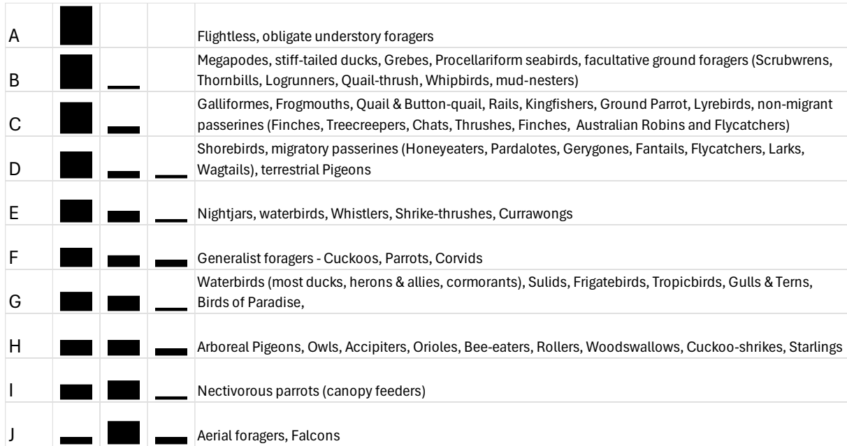
Figure 3. Flight height grouping for Australian birds. The relative height of the bars is illustrative of the relative amount of time that birds in this trait group are expected to fly below, within and above collision risk height (i.e., within the area encompassed by the rotating blades)
