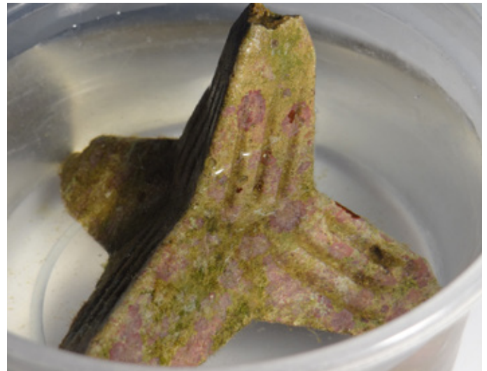
Figure 26: Biofilm on a concrete unit (photo: SECORE).
