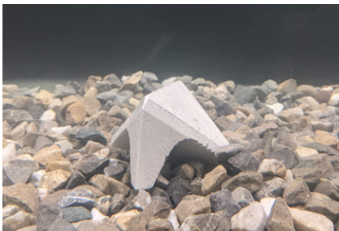
Figure 70 & 72: Orientation of 'Mich. idee' in a high flow velocity.
