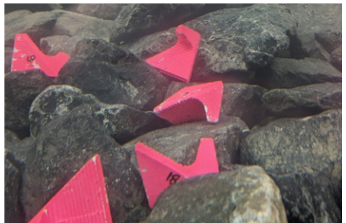
Figure 69 & 71: Orientation of 'Driehoekpaal' in a high flow velocity.
