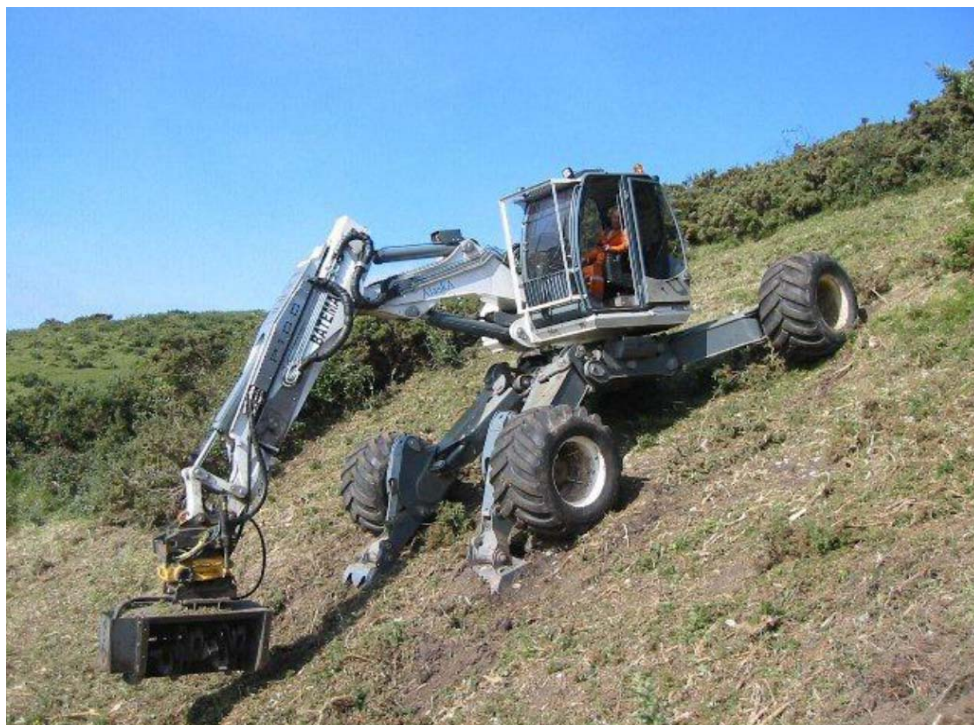
Figure 2b.13: Batemag Machine with Cutting Head (Alaska Environmental Contracting Ltd)
