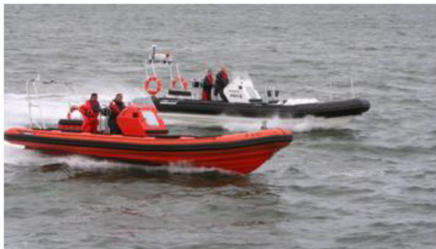
Figure 2a.20: Typical RIB for ferrying passengers and small tools and equipment in very calm sea conditions
