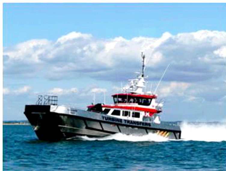
Figure 2a.19: Typical service vessel which can carry 12 passengers and equipment, approx 18x7m
