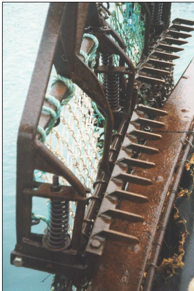
Figure 18.49 A Springer dredge illustrating the Spring Retained Tooth Bars
