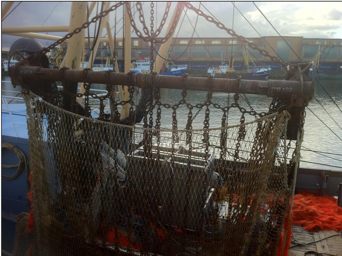
Figure 18.62 Belgian Beam Trawl as used in the ROWF are with Chain Mat Fitted (Source: BMM, 2011).
