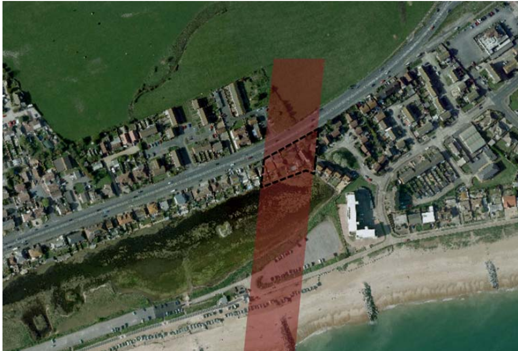
Figure 2: Potential landfall location at eastern end of Widewater Lagoon, showing indicative HDD corridor requirement (red)
