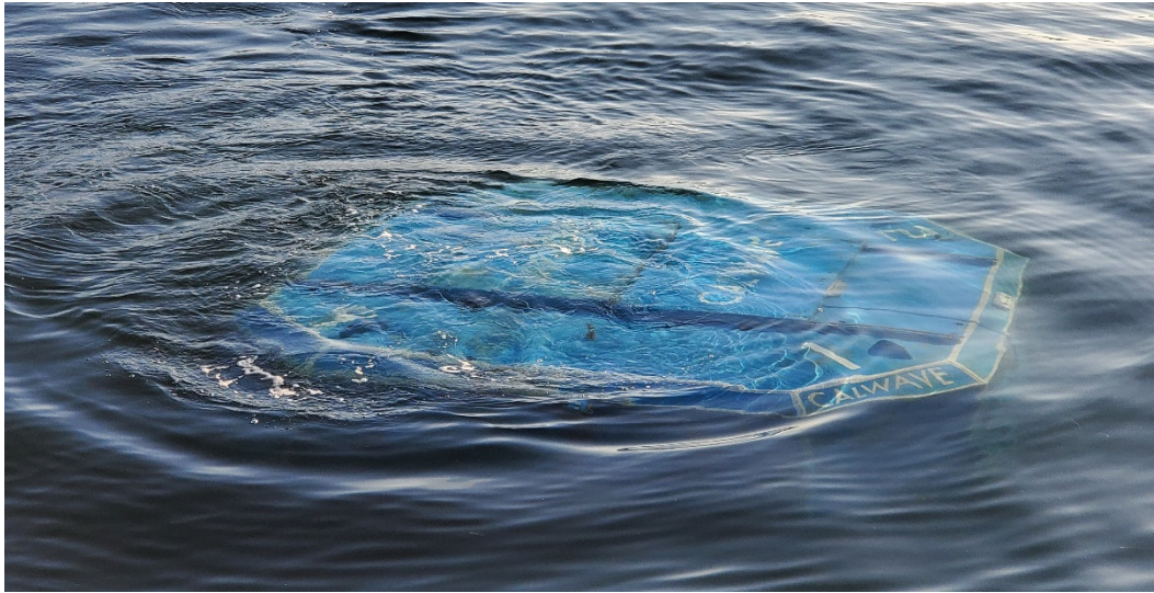
Figure 32. CalWave device at sea surface with hatch closed.
