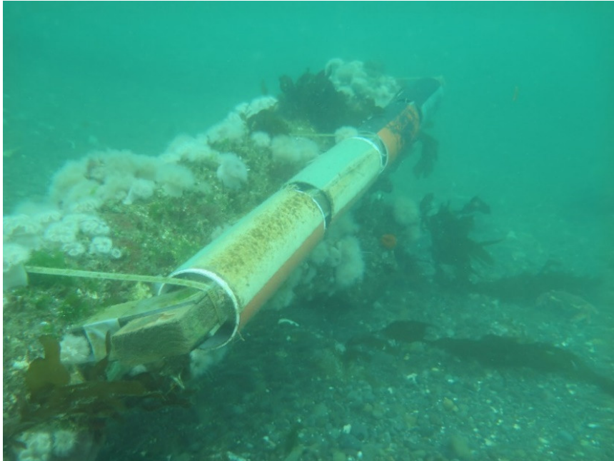
Figure 7. Flow noise shield biofouling test setup.
