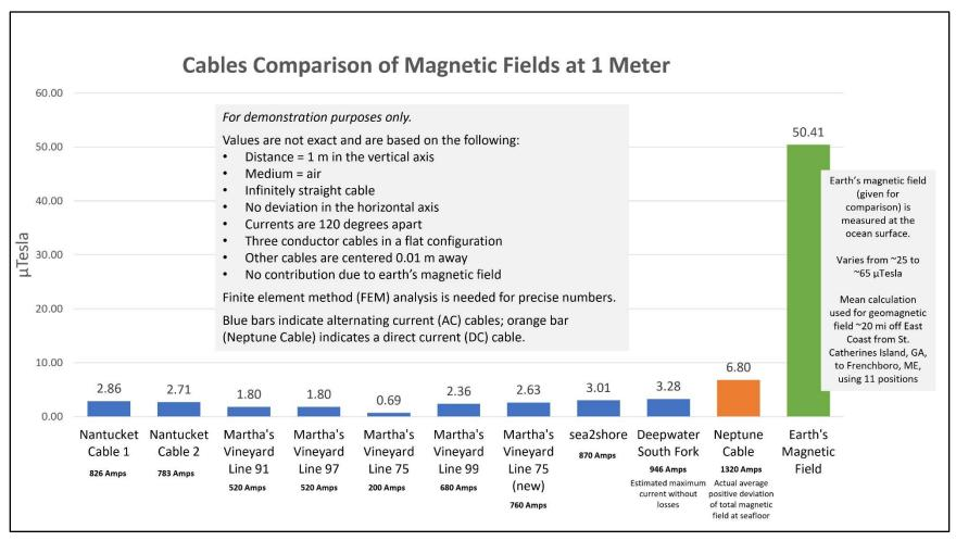
Figure G-EMF1. Comparison of electromagnetic fields produced by offshore wind farm transmission cables to the Earth's background magnetic field.
