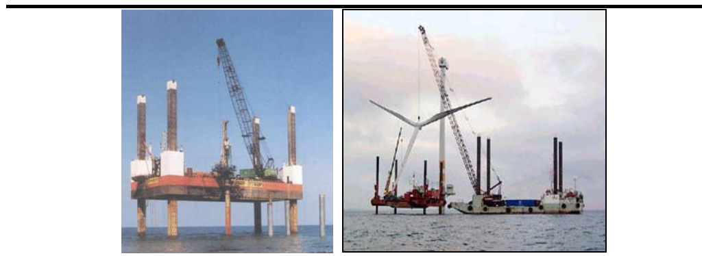
Figure 3.6 Photographs of Typical Jack-up Barges (Courtesy of Hydrosol Services (left hand picture) and Enron Wind (right hand picture))
