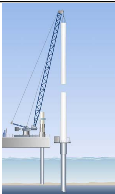
Figure 3.8 Illustration of the Tower Installation (Courtesy of Enron Wind)
