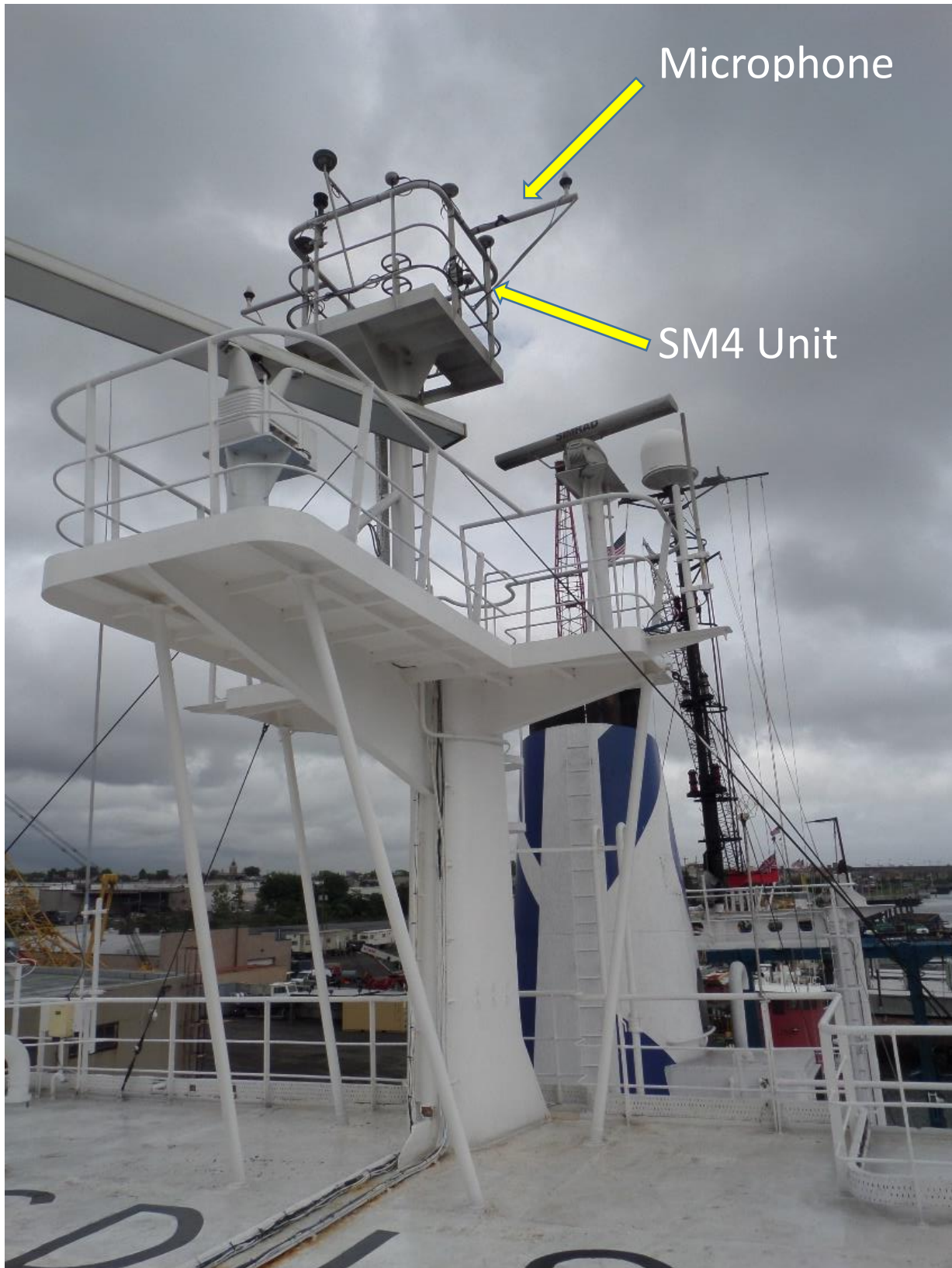
Image 2 Location of the Microphone and SM4 Unit on the Research Vessel Ocean Researcher
