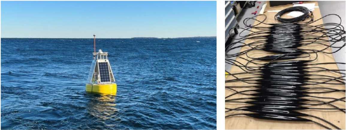
Figure 2 SeaPicket system: (a) Surface buoy with satellite comms and solar panels, and (b) 32-channel hydrophone array
