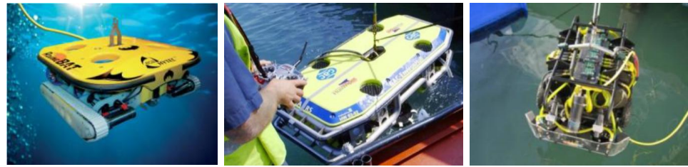
Figure 4. ROV for cleaning with partial inspection function [48].
