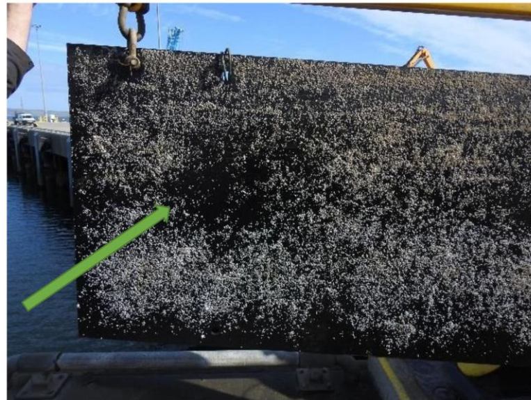
Figure 5. Biofouling being removed with an HPUT, with the green arrow indicating the HPUT's position behind the plate [67].
