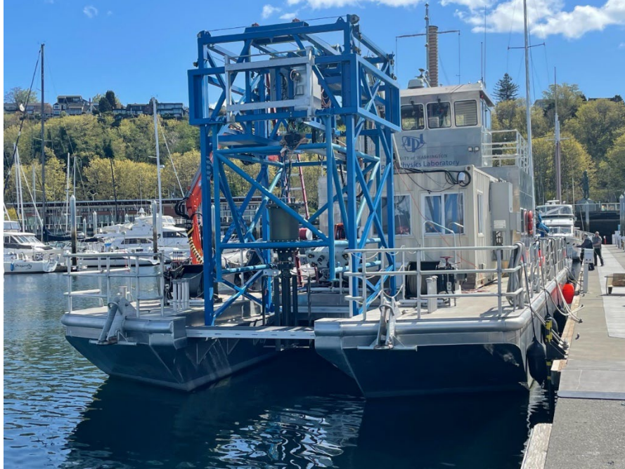
Figure 2: A picture of the Turbine Lander rotor and PTO installed on RDL prior to testing in Agate Pass, WA.
