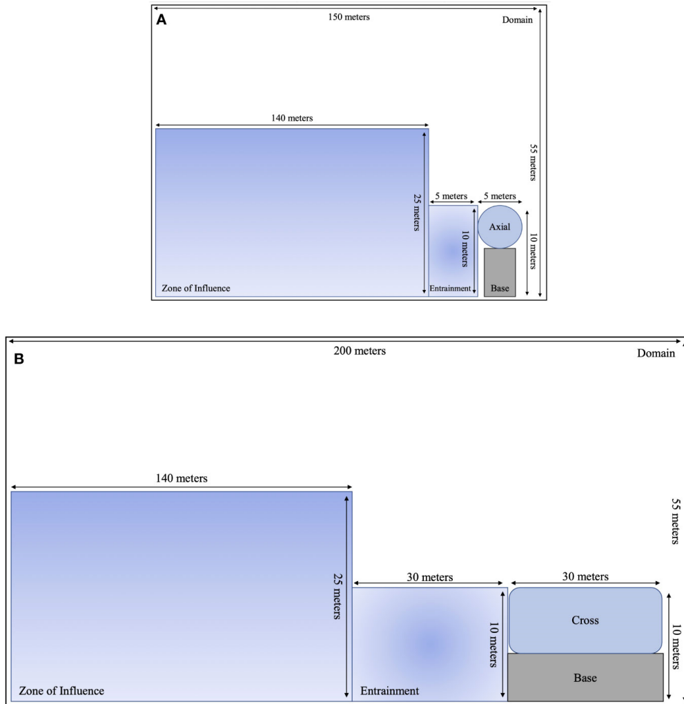
Figure 54. A two-dimensional schematic showing dimensions of the encounter-impact model components for (A) axial and (B) cross-flow turbines.
