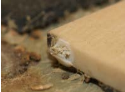
Figure 2.1 – Barnacle attached to edge of glass fiber composite sample
