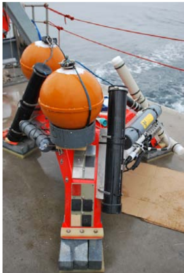
Figure 1.1 – Material samples attached to instrumentation tripod
