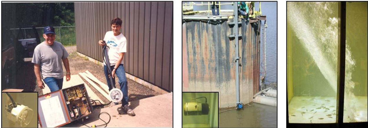
Figure C-4. Behavioral barriers that have been shown to be biologically effective for particular species. From left to right: strobe lights, sound transducers, and air bubble curtains.
