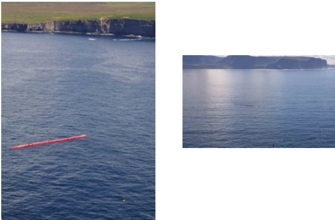
Figure 4. Example of the Visibility of a Low Freeboard High Color Contrast WEC Device
