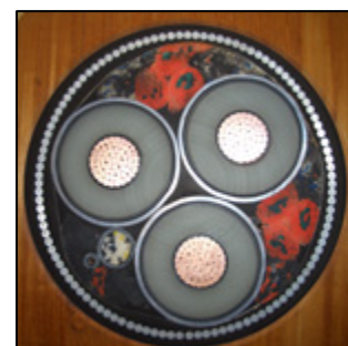
Figure 3. Cross section of LIRC Cable.
