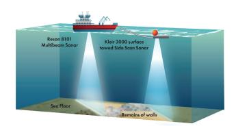
Credit: BOEM. Geological and Geophysical Surveys. 2018. Examples of geophysical survey equipment include multibeam echo sounders and side scan sonars
