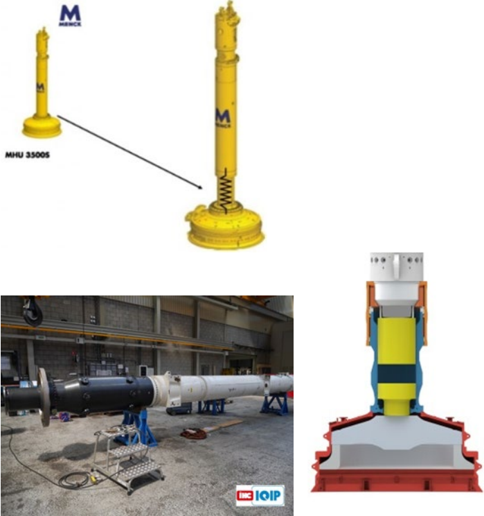
Fig. 7. View of a standard hydraulic impact hammer and a modified hammer (right) with a MENCK Noise Reduction Unit (MNRU) added between ram weight and anvil (left, © MENCK) and IHC S-90 hammer with added PULSE system in black housing (middle) and cross-sectional view (right, © IHC IQIP).
