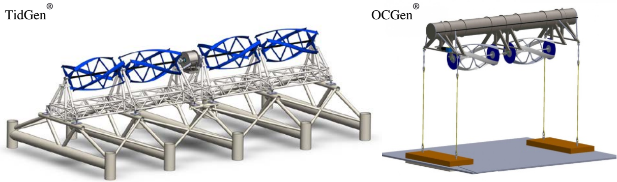
FIGURE 2 Schematic representation of the TidGen (9.5×31.2×15.2 m) and OCGen (5.1×19.7×5.3 m) power systems that ORPC installed in outer Cobscook Bay, Maine. Only the bottom mount of the TidGen system was present during the 2014 mobile hydroacoustic fish surveys over the OCGen power system (Source: Shen et al. 2016).
