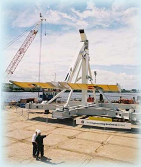
Oscillating Hydrofoil (Stingray) Source: The Engineering Business
