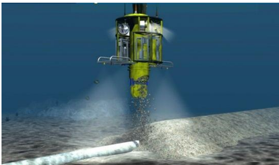
Figure 15: Example rock berm (Nordnes, 2017).
