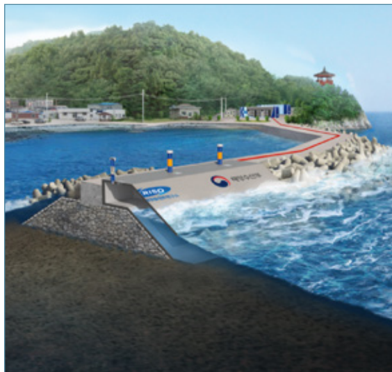
WEC applicable to breakwaters on remote island
