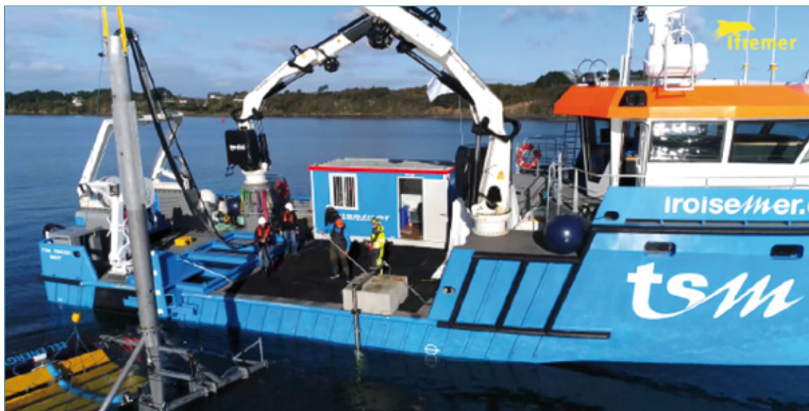
Set-up of the Eel Energy membrane for the tests in the Brest harbour – Copyright Ifremer
