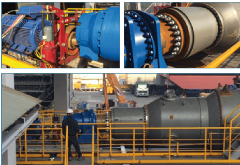
Dynamo test for PMSG and drive train of 200 kW TEC
