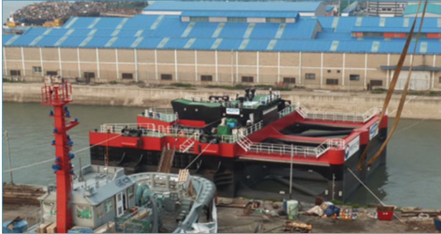
300 kW Floating pendulum wave energy converter in port
