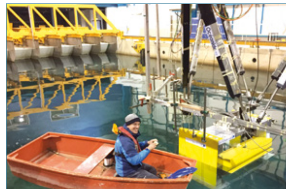
Floating Power Plant testing a section of its wave energy model
