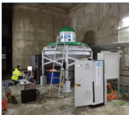
Model testing of the twin-rotor air turbine (left) at IST; biradial turbine prototype installed at the OWC-breakwater, Mutriku, Spain (right).
