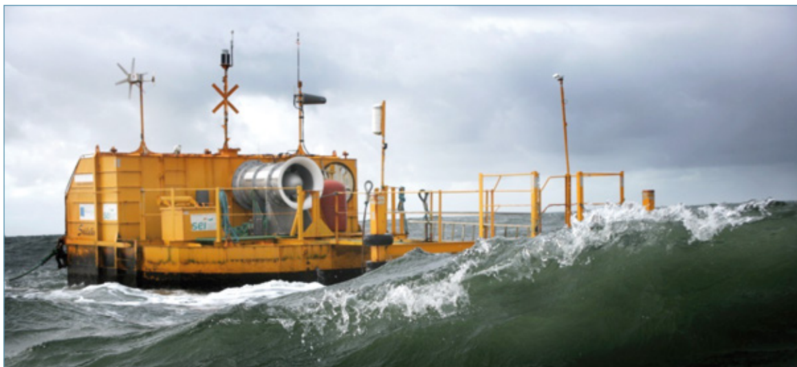
Ocean Energy Buoy in Galway Bay Marine Renewable Energy Test Site
