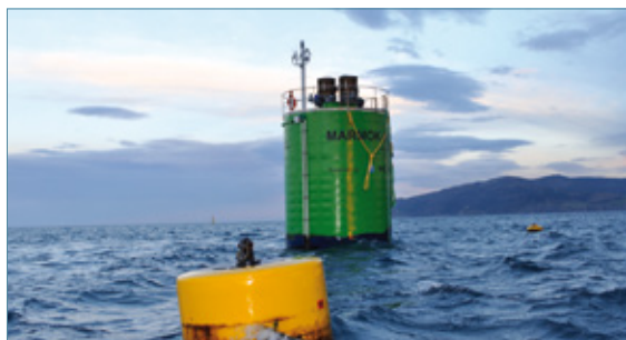
MARMOK-A-5 wave energy device at BiMEP
