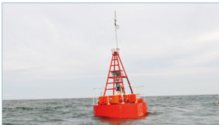
Testing of NIOT's wave powered navigational buoy near Kamarajar Port, Chennai
