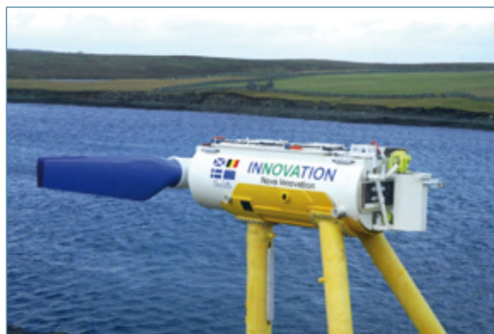
Nova M100 turbine, installed in the Shetland Tidal Array (Source: Nova Innovation)
