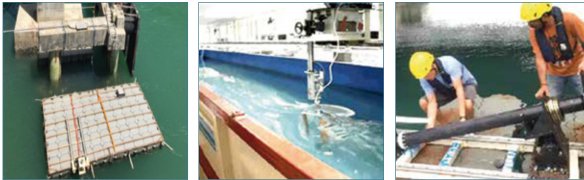
Floating hinged turbine support frame to house tidal turbine devices(Left), Scaled (1:3) tidal turbine in tow tank (Middle) and successful deployment of the turbine at Sentosa Test site. (Right)
