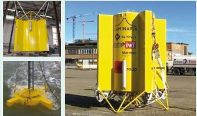
1:5 scale model of the Laminaria WEC while testing the height adaptation (top left), before open ocean testing (right) and during testing (down left).
