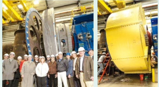
Representatives from Columbia Power Technologies, NREL and project partners at NWTC facilities at the project start (left), generator connected to the 5 MW dynamometer (right). Courtesy: Mark McDade, NREL
