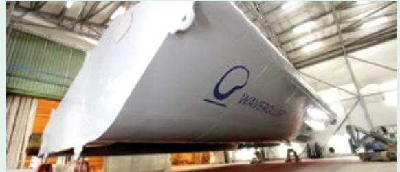
WaveRoller® 3 x 100 kW demonstration in Peniche in 2012 (top) and new panel for the commercial size 350 kW unit (down). Courtesy: AW-Energy
