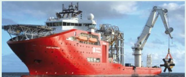
D10 device installation (top) and recovery of the turbine (down). Courtesy: SABELLA
