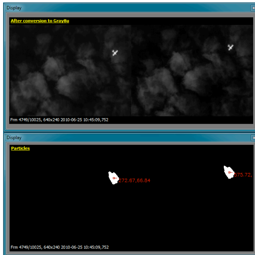
Figure 3–53. Thermal imagery (above) and filter-detected objects (below) from 100 m flyover test.
