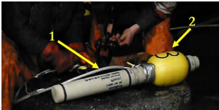
The new T-POD attachment. Kevlar cable with rubber tubing (1) and buoy (2) for additional buoyancy.
