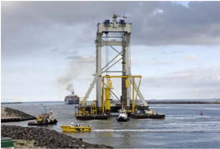
Photo: the Svanen going out with monopile and transition piece on board.
