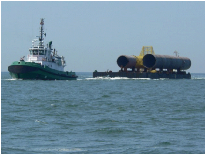
Monopile and Transition piece on transportation barge, one set per barge.
