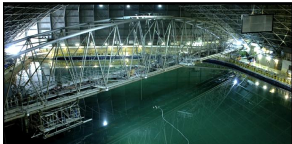
Figure 7. Curved Corner of EDL 216 Paddle Directional Wavemaker
