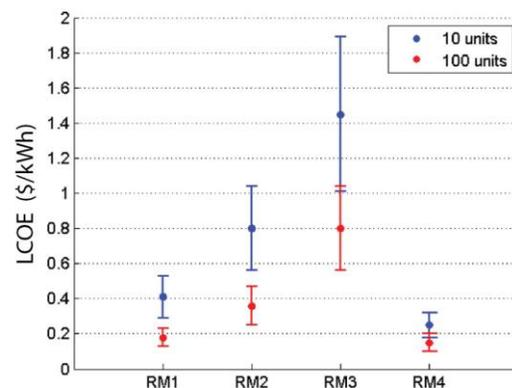
**Figure 3. LCOE estimates for four reference MEC technology point designs.**
